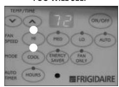
Note: Remember that in this mode, the fan will run continuously while the compressor cycles on and off as needed to maintain the room temperature. (See also, power saver mode, step 6)
